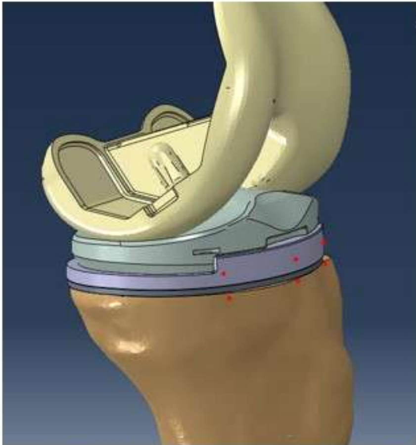
Figure 1. Cadaveric Micromotion Measurement Points
