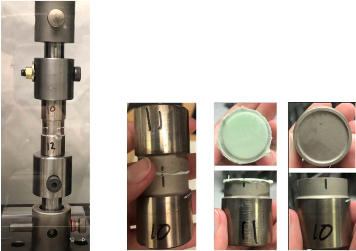
Figure 1. Left: Instron jaw setup. Right: Successful coupon break condition.
