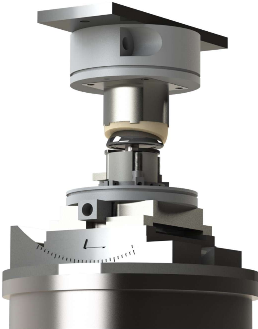
Figure 2: A render showing a closeup of the fixtures. Micromotion fixtures are attached to bone substitute, and lubricant can be circulated through polymer components. An angled component allows for the glenoid version angle to be altered.
