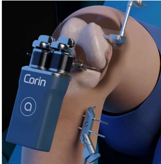
Figure 1: A ligament tensing device which allows for soft tissue assessment prior to bone resections.
