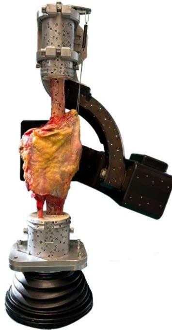
Figure 1. Experimental setup with an instrumented knee specimen mounted on the six-degrees-of-freedom joint motion simulator at 0° flexion.
