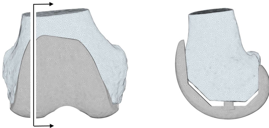
Figure 1: On the left, the cutting plane in the coronal plane through the lateral condyle is shown. The cross sections in this article display the perspective towards the center of the femur. On the right, the simulation of the implant pull-off is shown.
