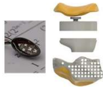
Fig 1C. The underside of the distal component of the Diaphragm design instrumented with 5 strain gauges (L). An exploded view of the components of the Diaphragm design: distal articulating surface, diaphragm, container, and trapezium body with proximal articulating surfaces (R, top to bottom).
