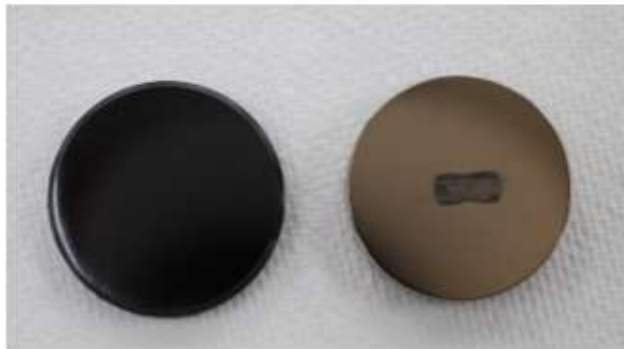
Figure 1: Representative images of OxZr (left) and TiN coated Ti6Al4V (right) disks after testing.
