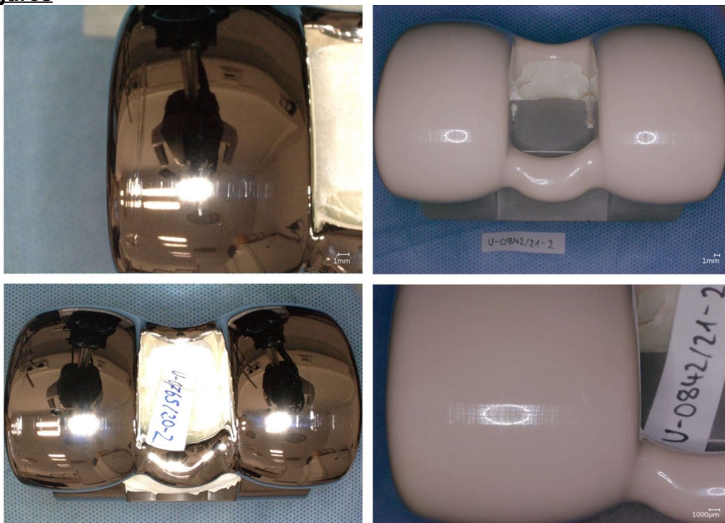
Figure 1: Vega System® PS femoral component in CoCr28Mo6 (left) and made out of PEEK-OPTIMA™ (right) after 5 million HDA knee wear test cycles with slight scratches on the condylar bearing surfaces (both materials) and without any cracks or deformations on the cam of the PEEK femoral component
