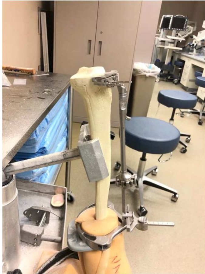
Figure 2. Bone model in conventional closed extramedullary tibial resection guide setup for cutting.
