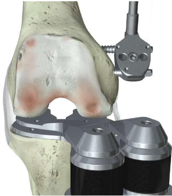
Figure 1: A robotic ligament tensioner collects laxity data before and after PCL resection.
