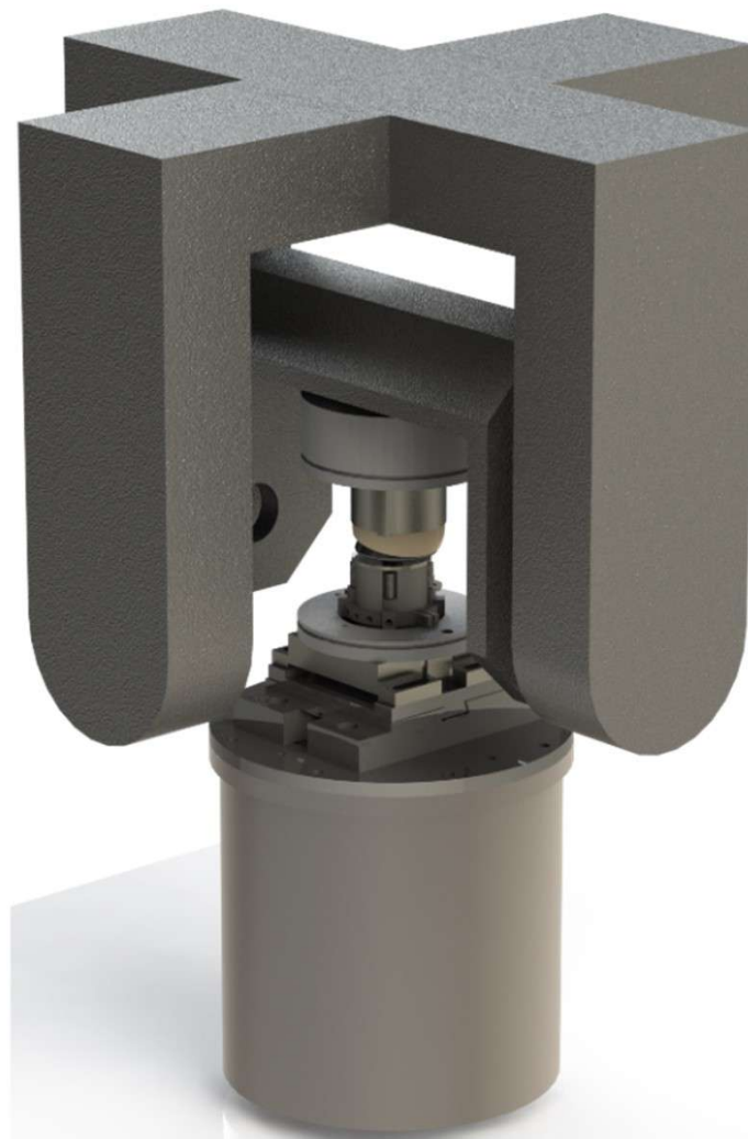
Figure 1: Rendering of the apparatus. The superior rockers can be orientated with respect to the component to apply flexion and abduction in the ideal plane. The inferior plate rotates to apply axial rotation.
